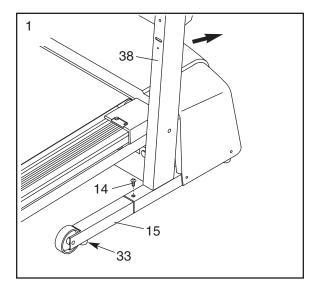
Insert the tab on one of the Handrail Brackets (17) into the slot in the right Upright (38). Attach the Handrail Bracket with a 3/4" Screw (5) and a Star Washer (25). Attach the other Handrail Bracket to the left Upright (not shown) in the same way.
